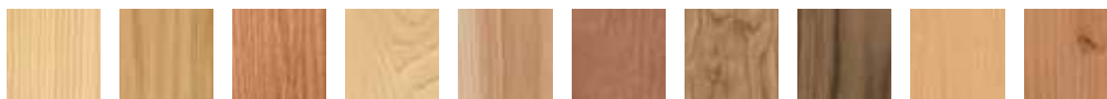
Pine Mixed Grain Douglas Fir Oak Maple Hickory Mahogany* Cherry Walnut Vertical Grain Douglas Fir Alder
